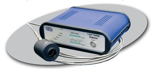
The **Laser Timing Stabilizer** consists of a fiber coupling mechanics which is mounted directly at the laser exit. A stable optical fiber leads the collected light to a controller where a fast photodiode measures the inherent time separation of the laser pulses.
