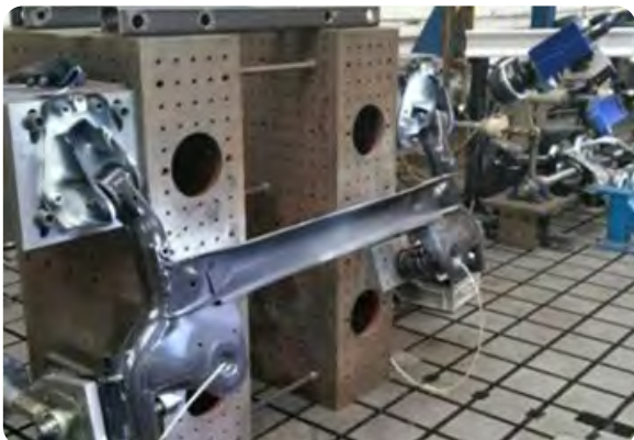
Measurement of sub frame joints
